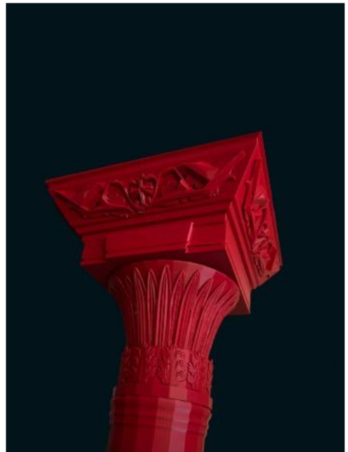
Figure 2. Printed Model with FlashForge Adventurer 5MPro and HS-PLA Ruby Red 1,7mm filament.
